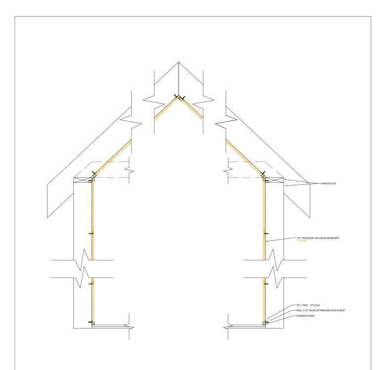
$^1$  Allow a minimum of  $\frac{1}{16}$ " gap between the back of the screw and the head of screw flange. Screw should penetrate a minimum of 1" into solid backing.
