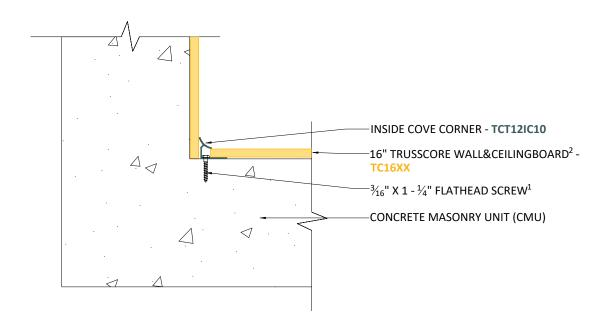
$^{1}$  Allow a minimum of  $\frac{1}{16}$ " gap between the back of the screw and the head of screw flange. Screw should penetrate a minimum of 1" into solid backing.
