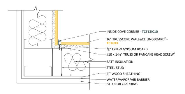
$<sup>^1</sup>$  Allow a minimum of  $\frac{1}{16}$ " gap between the back of the screw and the head of screw flange. Screw should penetrate a minimum of 1" into solid backing.
