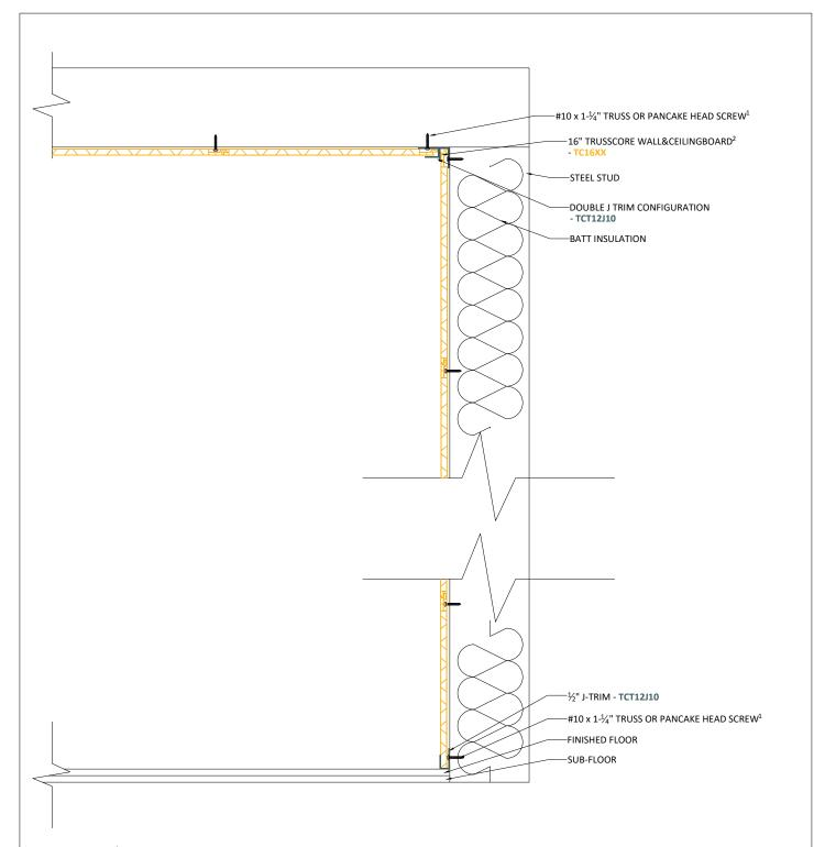
$<sup>^1</sup>$  Allow a minimum of  $\frac{1}{16}$ " gap between the back of the screw and the head of screw flange. Screw should penetrate a minimum of 1" into solid backing.
