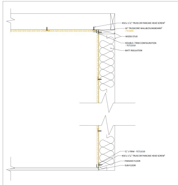
$^1$  Allow a minimum of  $\frac{1}{16}$ " gap between the back of the screw and the head of screw flange. Screw should penetrate a minimum of 1" into solid backing.
