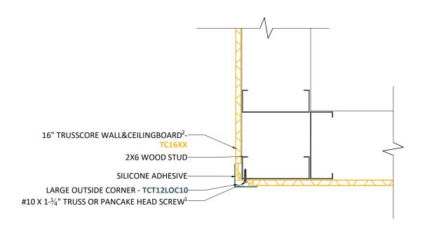
$^3$  Outside Corner Square trim is intended to be adhered to Wall&CeilingBoard with a one-part, neutral cure silicone sealant.
