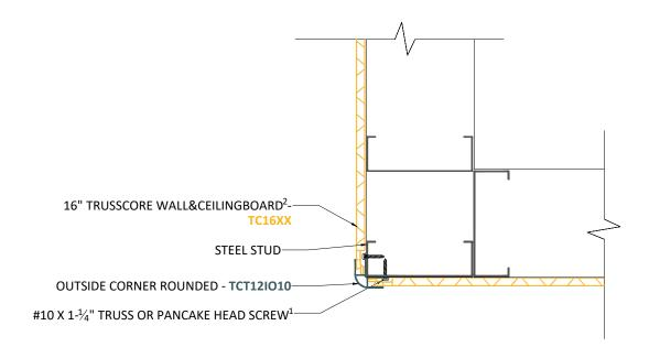
$<sup>^1</sup>$  Allow a minimum of  $\frac{1}{16}$ " gap between the back of the screw and the head of screw flange. Screw should penetrate a minimum of 1" into solid backing.
