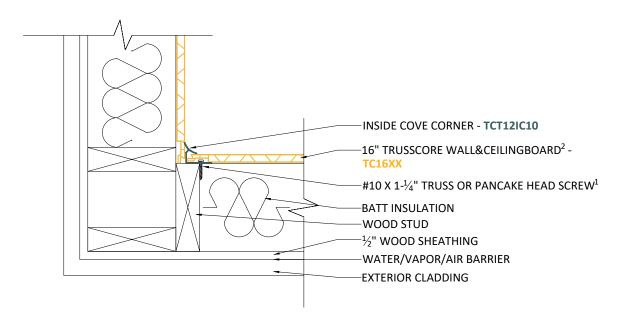
$<sup>^{1}</sup>$  Allow a minimum of  $\frac{1}{16}$ " gap between the back of the screw and the head of screw flange. Screw should penetrate a minimum of 1" into solid backing.
